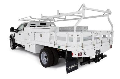
Contractor body comes equipped with many of the features that customers expect from Reading Truck, including A60 galvannealed steel construction, e-coat primer and powder coat finish. "Contractors are demanding a better-equipped and more flexible work truck, and we believe that we have met that challenge." said McNally.
